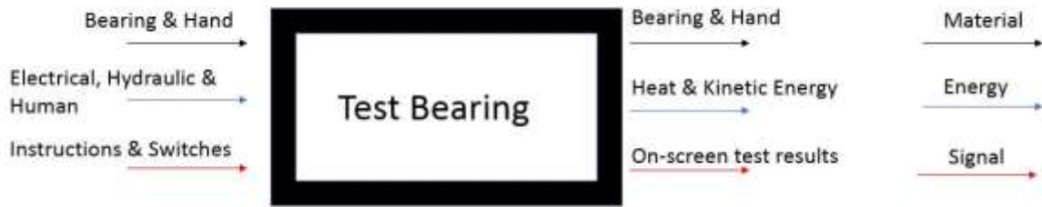
Figure 5: Black Box model for Testing Bearing
